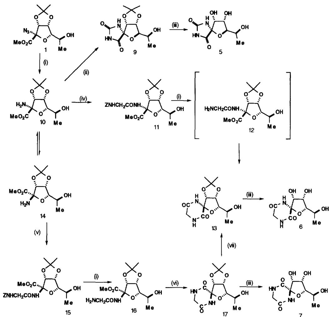
**Scheme:** (i)  $H_2$ , Pd black, EtOH (ii) KCNO, MeCOOH (iii) 50% aq.  $CF_3COOH$  (iv) ZglyOH,  $ClCOOEt$ ,  $Et_3N$ , THF; pyridine, MeCN (v) ZGlyOH, DCC, 1-hydroxybenzotriazole, DMF (vi) MeOH (vii) *tert*-BuOK, DMF
